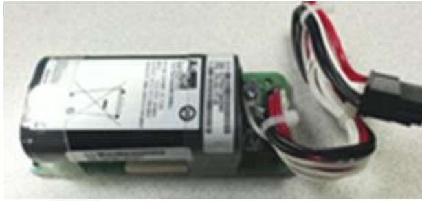
Figure 6. Battery backup unit
