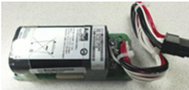
Figure 15. Battery backup unit
