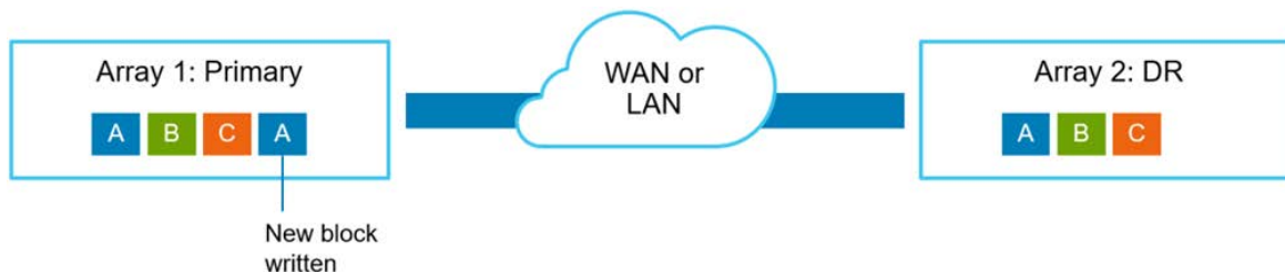
Figure 1. Conventional Replication: Non-Unique Block "A" Added to Array 1
