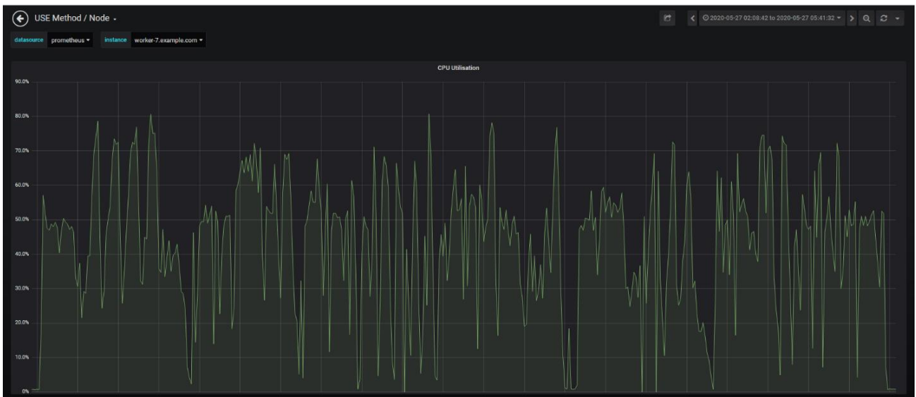
Figure 4 Worker node CPU utilization in the OpenShift Grafana dashboard
