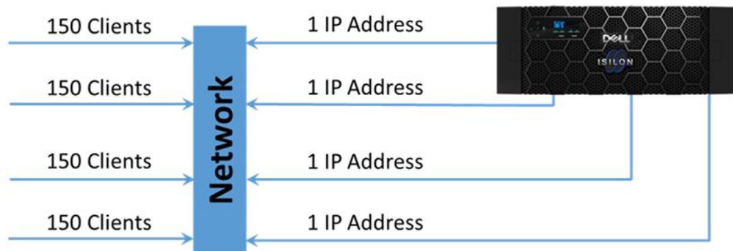
Figure 11. Dynamic allocation: Four-node cluster with one IP address per node
