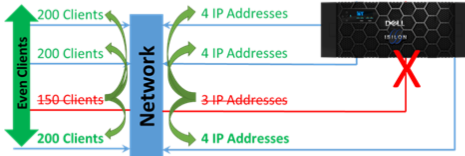
Figure 14. Dynamic allocation: Four-node cluster with two IP addresses per node, one node offline
