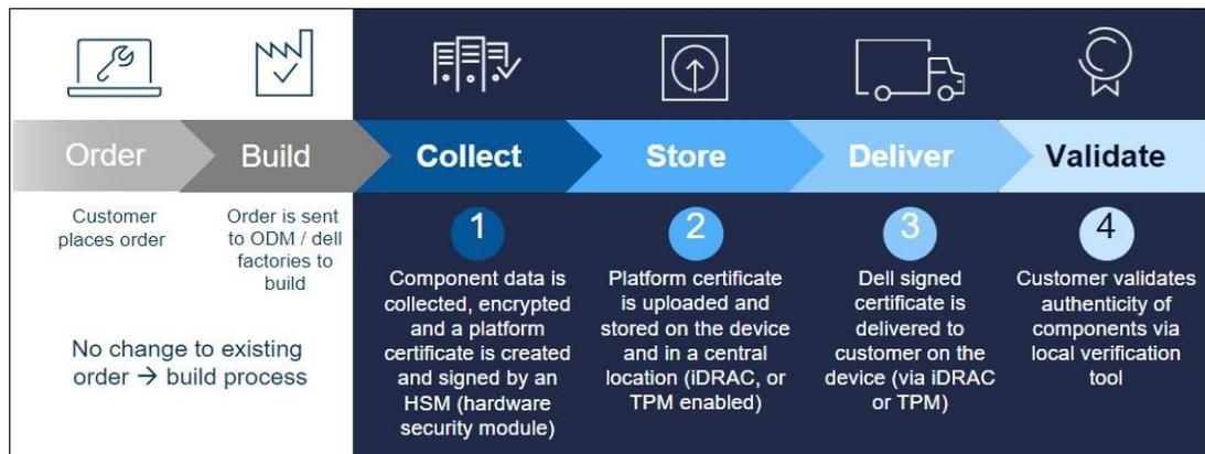
図3. Dell Secured Component Verification (SCV)
