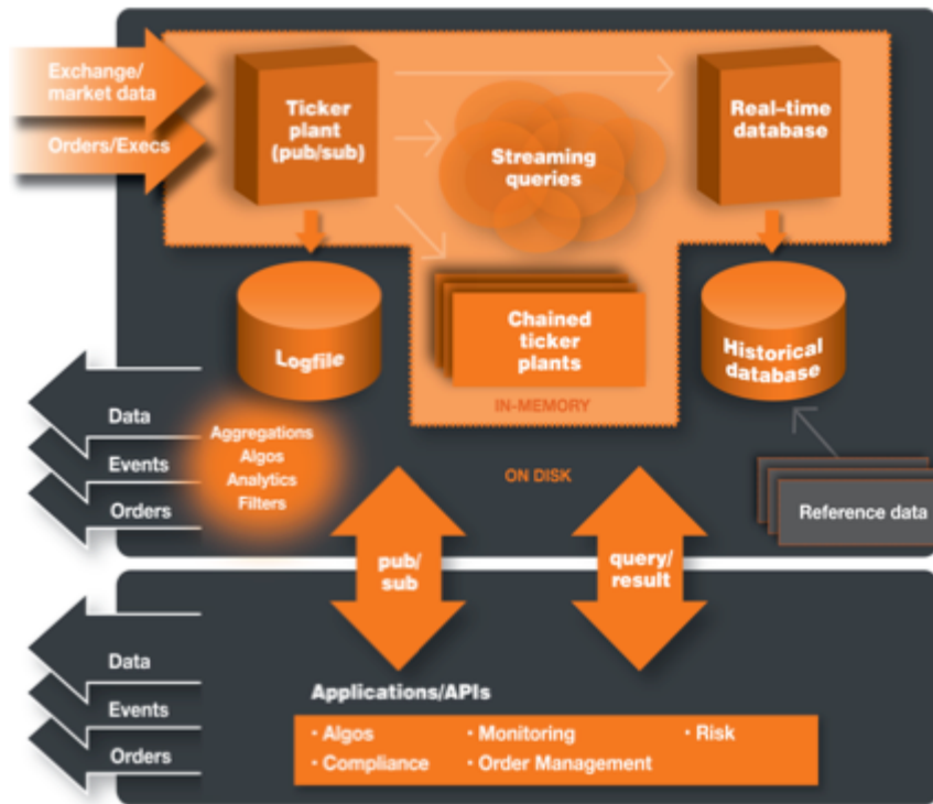
Figure 1: View of kdb+ system architecture
