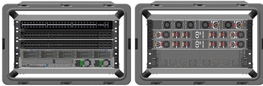
Figure 31. Dell T-R640 in management transit case (front view and rear view)
