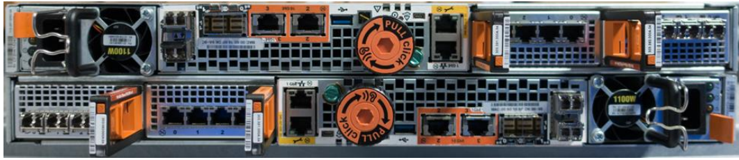
Figure 3. Rear of DPE (380/F)
