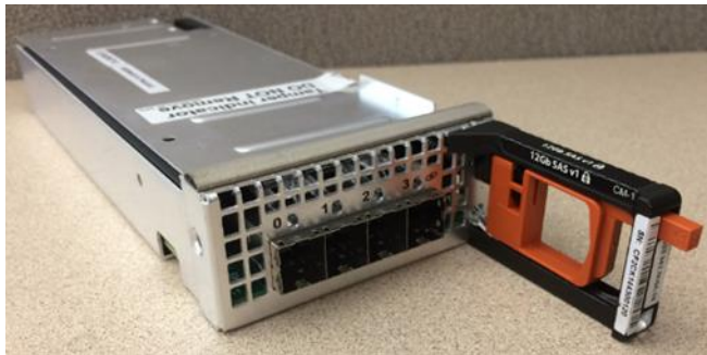
Figure 19. 12Gb SAS I/O Module
