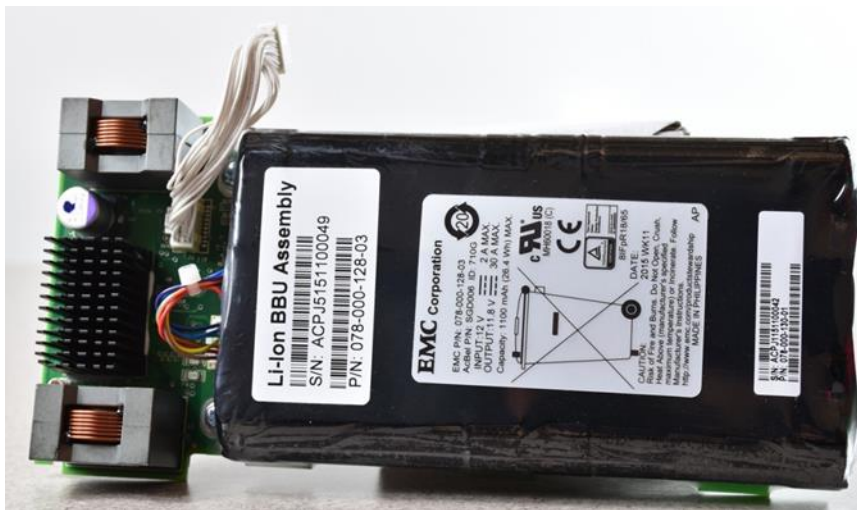
Figure 6. Battery Backup Unit (380/F)
