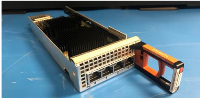
Figure 21. 10GbE BaseT I/O Module
