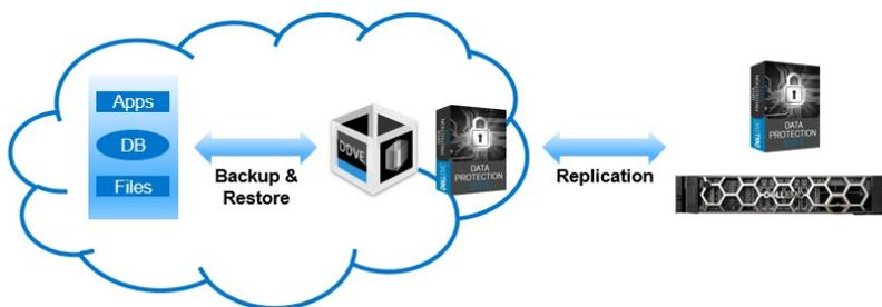
DDVE enables data protection in the cloud for applications running in the cloud. DDVE in the cloud allows for both backup and replication. Data can be moved to an on-premise DD series and backup to the cloud, or even backup and replicate data between two instances of DDVE running in the cloud or on-premise. This allows multiple DDVE instances to be spun up in other regions and backup and replicate the data over to keep everything consistent.
