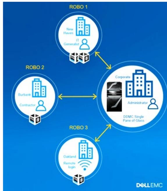
With a DD series appliance at the main data center and a DDVE at each branch office, you get the assurance that your data at these branch offices is protected. The entire data protection environment can be managed centrally with DDMC. If a branch office has a failure or must shut down, you have the peace of mind that the protected data is not lost. DDVE will divert that data into another remote office or stores it on-premises.
