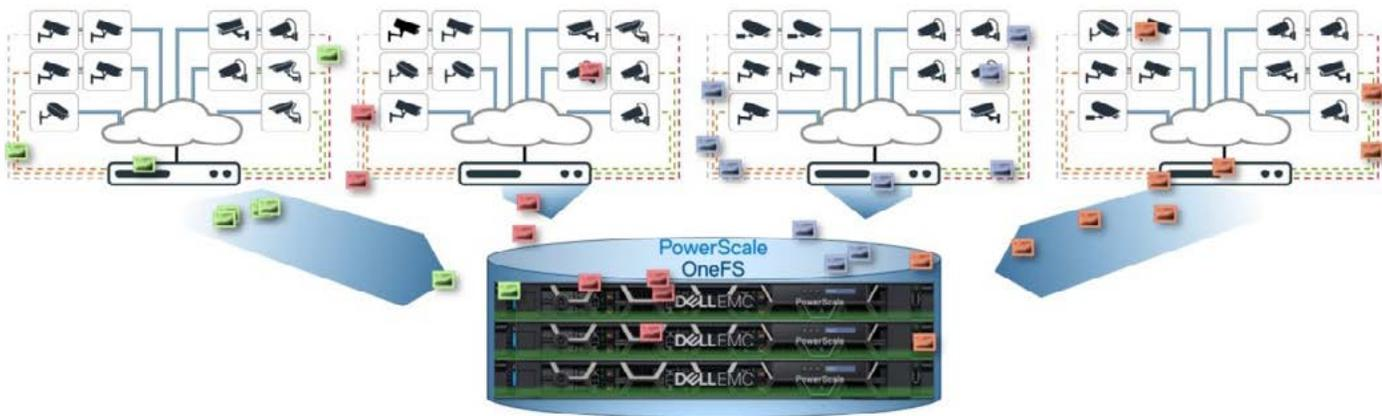
Figure 4: The distribution of safety and security traffic with a PowerScale cluster
