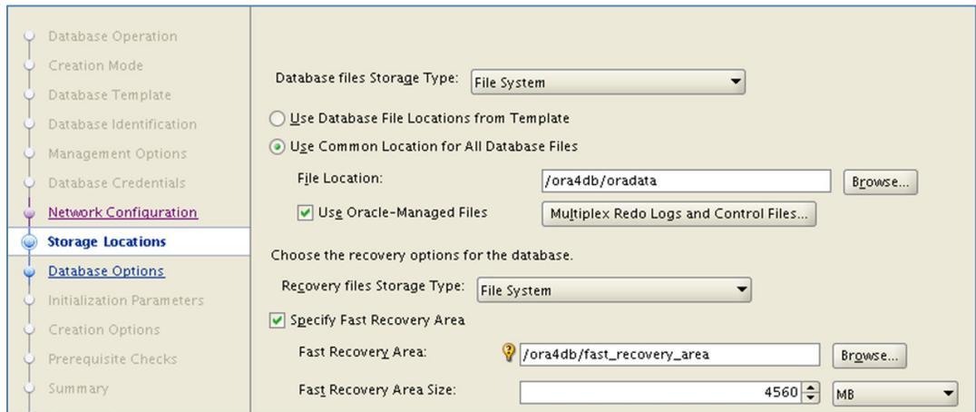
**Figure 13. Using file system for Oracle datafiles**
