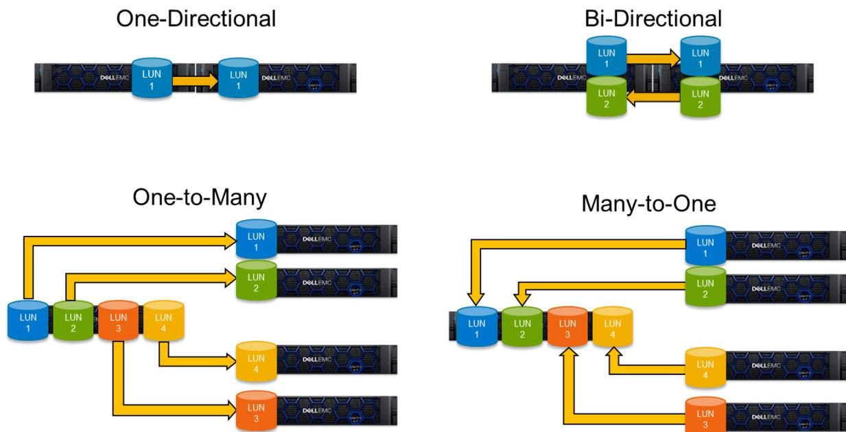
Figure 36 System level asynchronous replication topologies
