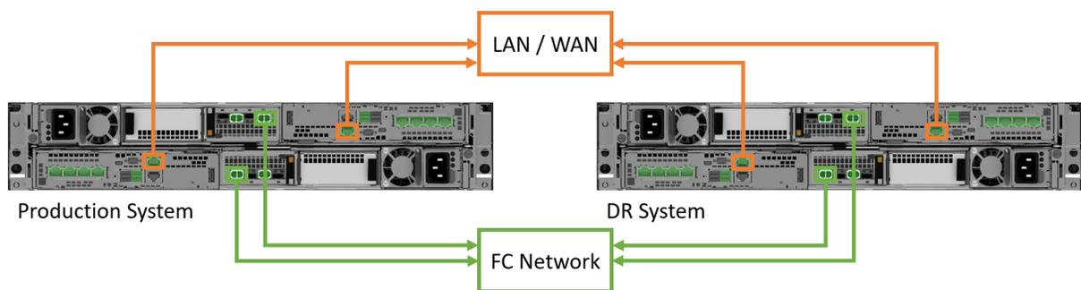
Figure 2 Native synchronous block replication connection example
