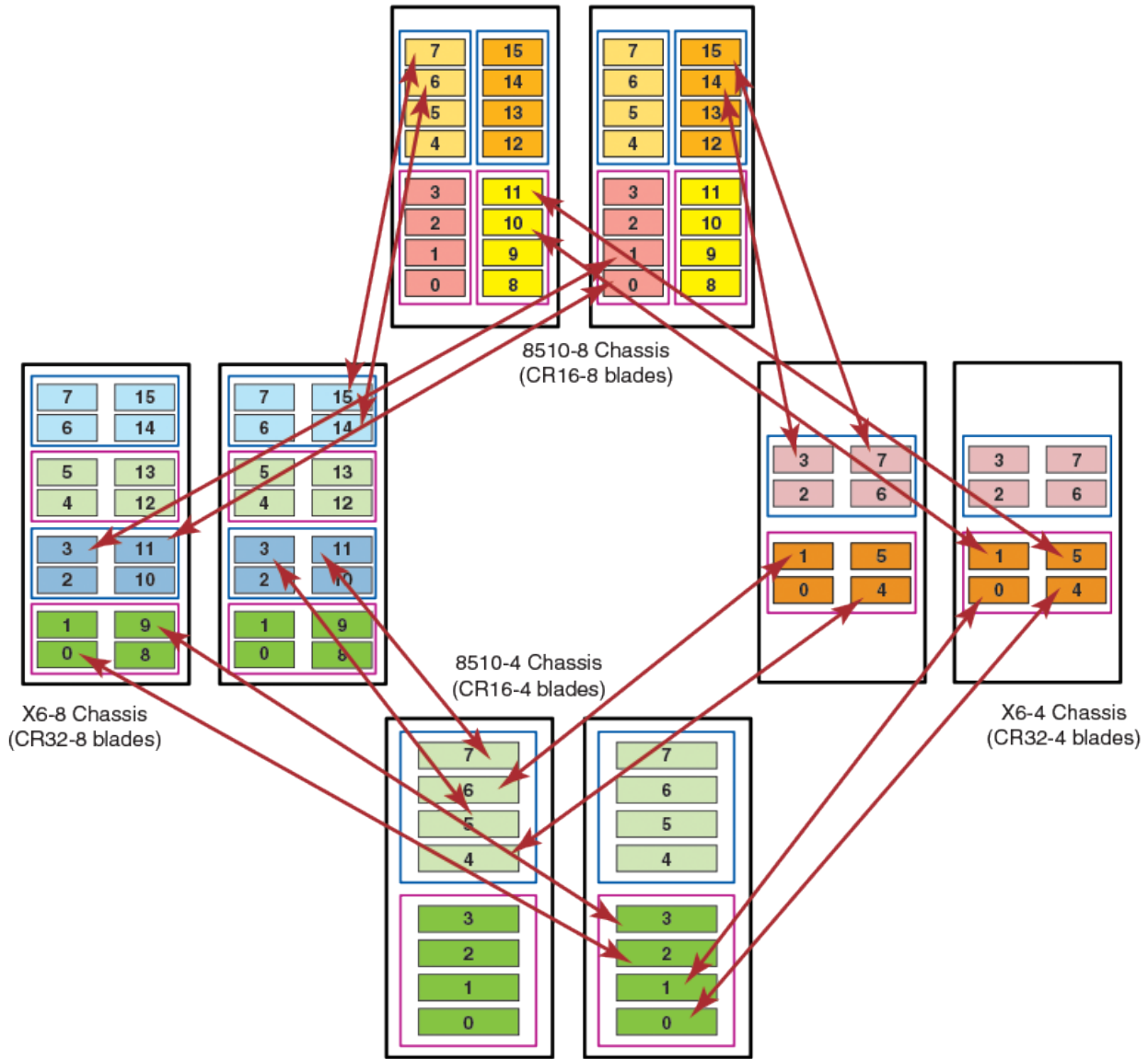
FIGURE 36 ICL trunks between DCX 8510 Backbones and X6 Directors
