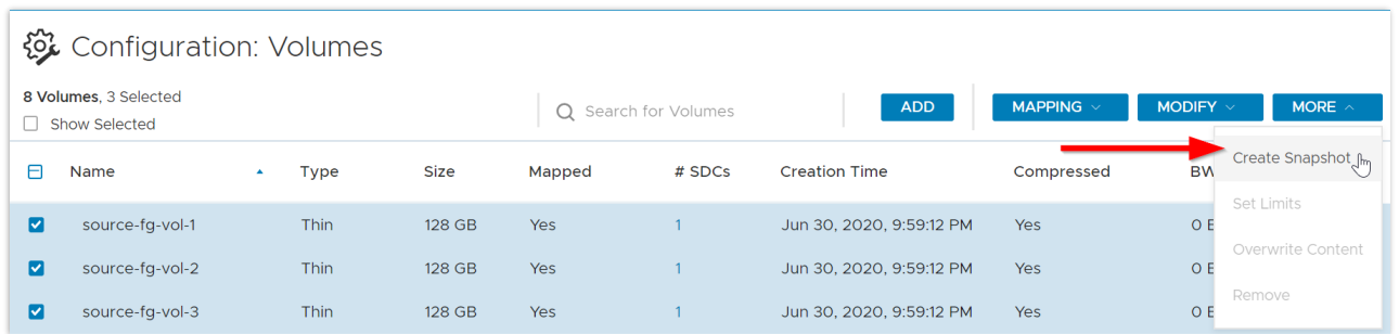
Figure 3 Creating snapshot of multiple volumes for snapshot consistency group
