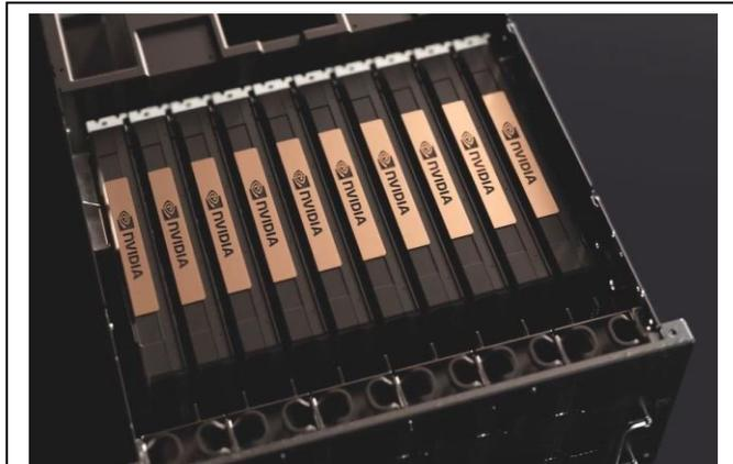
*NVIDIA V100 Tensor Core GPUs in the DSS 8440*
