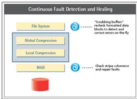
Figure 3. Continuous fault detection and healing protects against storage system faults. The system periodically re-checks the integrity of the RAID stripes and the container log and uses the redundancy of the RAID system to heal any faults. During every read, data integrity is re-verified and any errors are healed on the fly.
