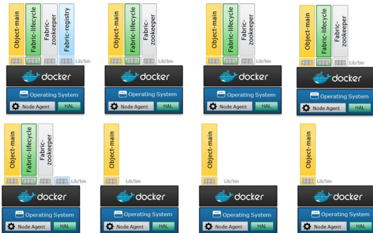
Figure 14. Docker containers and agents on eight node deployment example
