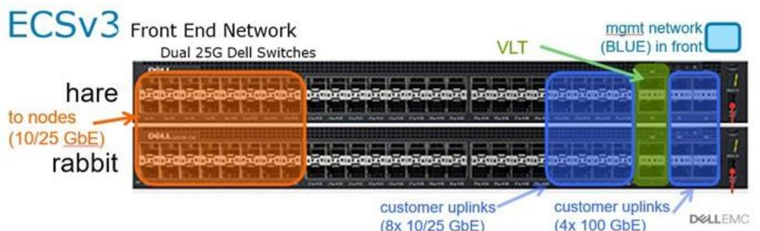
Figure 3 Front-end network switching in ECS deployment
