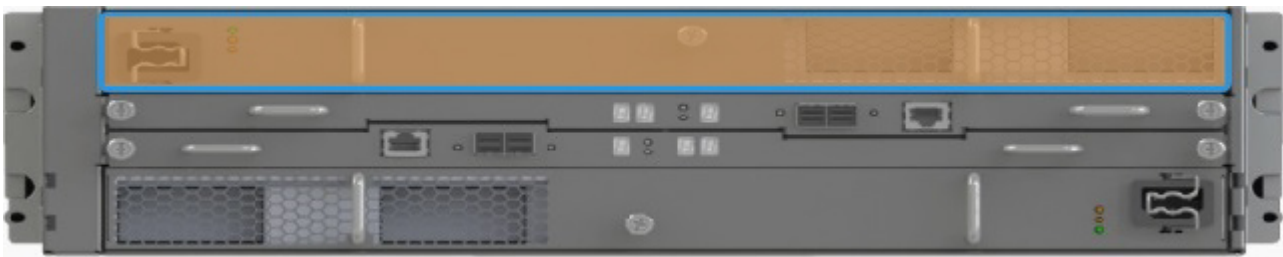
Figure 1 Faulted power/cooling module location - example
