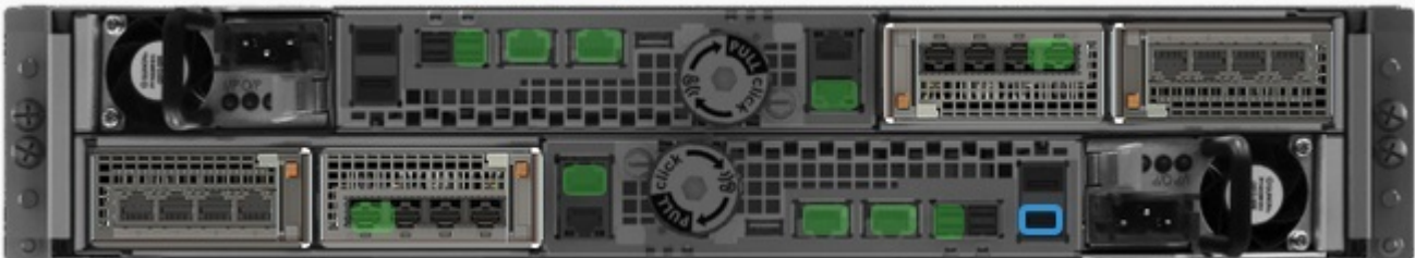
Figure 4 Healthy SFP in SP A port 4 - example location
