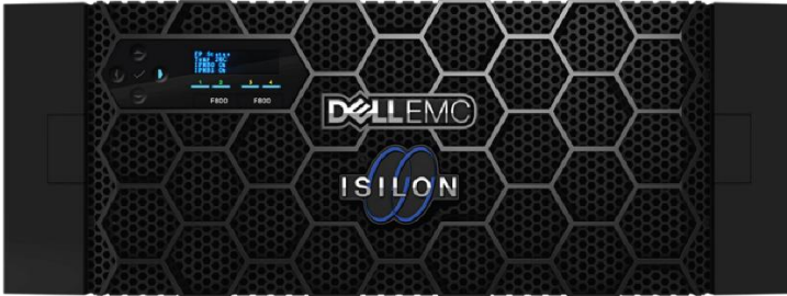
Figure 2 Isilon H500/F800 chassis, containing four storage nodes
