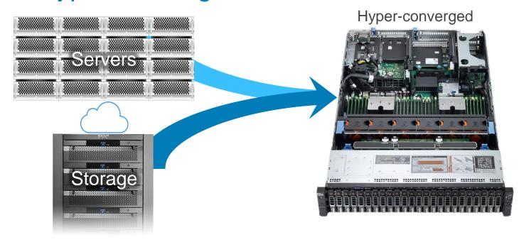
Hyper-converged infrastructure enables compute, storage and networking functions to be decoupled from the underlying infrastructure and run on a common set of physical resources that are based on industry-standard x86 components.\*
