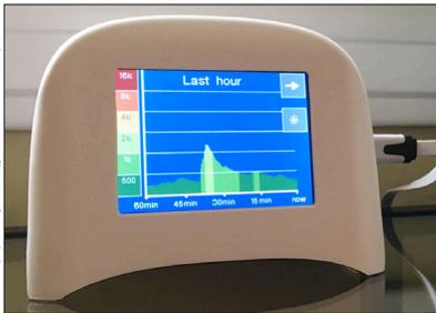
**Speck** is a Wi-Fi-enabled personal air quality monitor that measures the level of fine particulate matter in indoor settings.
