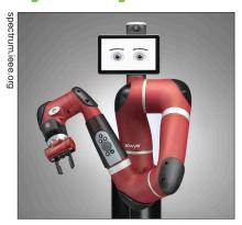
The user-friendly robot Sawyer learns by a human grabbing hold of its wrist and leading it through an activity once. Its series elastic actuators give it a high level of accuracy in sensing forces, enabling it to take on more delicate tasks.
