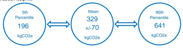
Carbon footprint calculations have a wide range based on a variety of factors including how the device is configured, where it was manufactured and more. Dell Technologies reports the 5th and 95th percentile of the carbon footprint estimate to reflect that uncertainty. For this product, that estimate has a mean of 329 kg of CO2e and standard deviation of 70 kg of CO2e.
