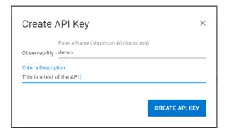
When the API key is created, the user selects the View Key link to obtain the Client ID and Client Secret. The user then uses these credentials to authenticate to a specific API endpoint to obtain an Access Token. When the user obtains the Access Token, the user can make the chosen REST API calls. The access token is active for one hour, and the client credentials are valid for one year.
