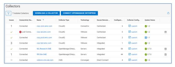
The user can select the hyperlink in the Name column to open the Collector Details page. This page provides health-related information for the selected collector. It also provides as an inventory of devices for which it is configured.
