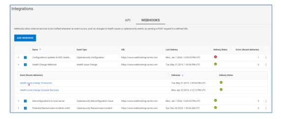
The user can select an event to see the Headers and Payload of the request and the response. A Redeliver button allows users to resend the event which is helpful for testing Webhook integration. Due to the potential sensitivity of cybersecurity information in the payload, users will only see header information in the Observability UI.
