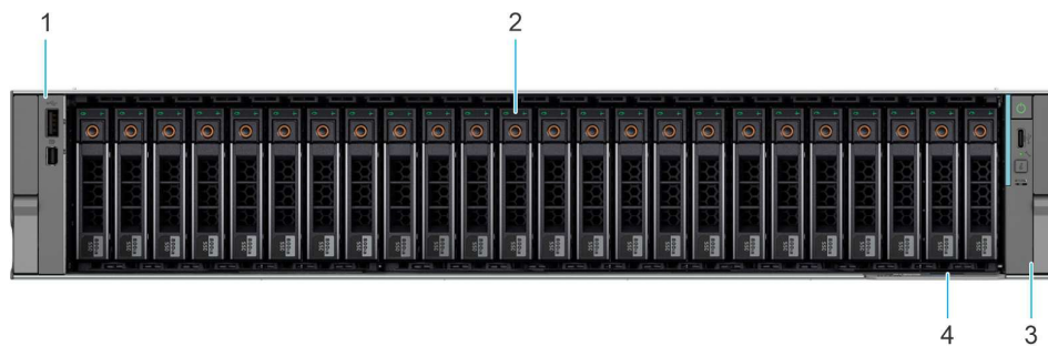
Figure 6. Front view of 24 x 2.5-inch drive system
