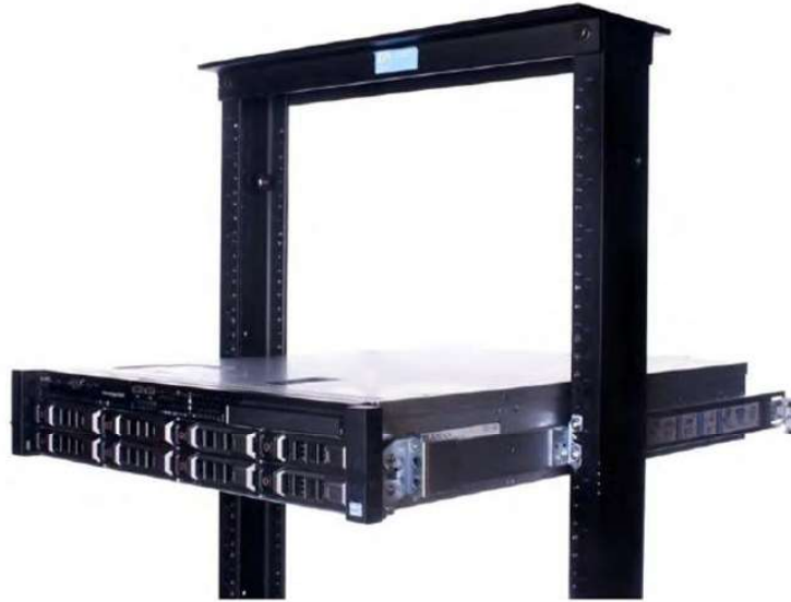
Figure 42. Static rails in 2-post center mount configuration
