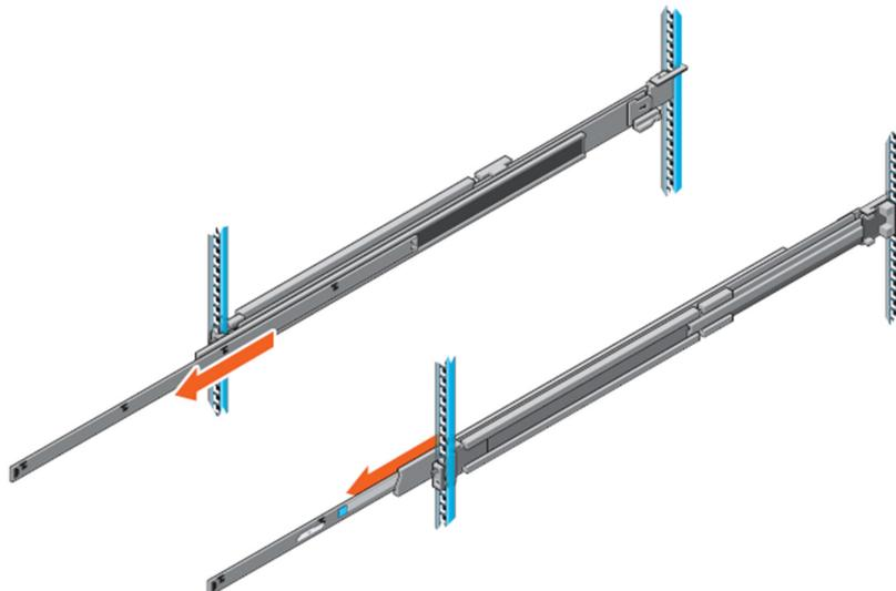
**Figure 29. Pull out inner rail**
