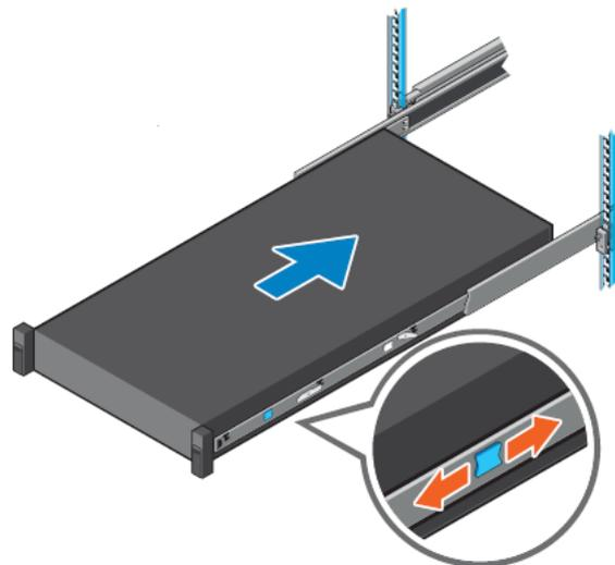
**Figure 31. Slide system into the rack**
