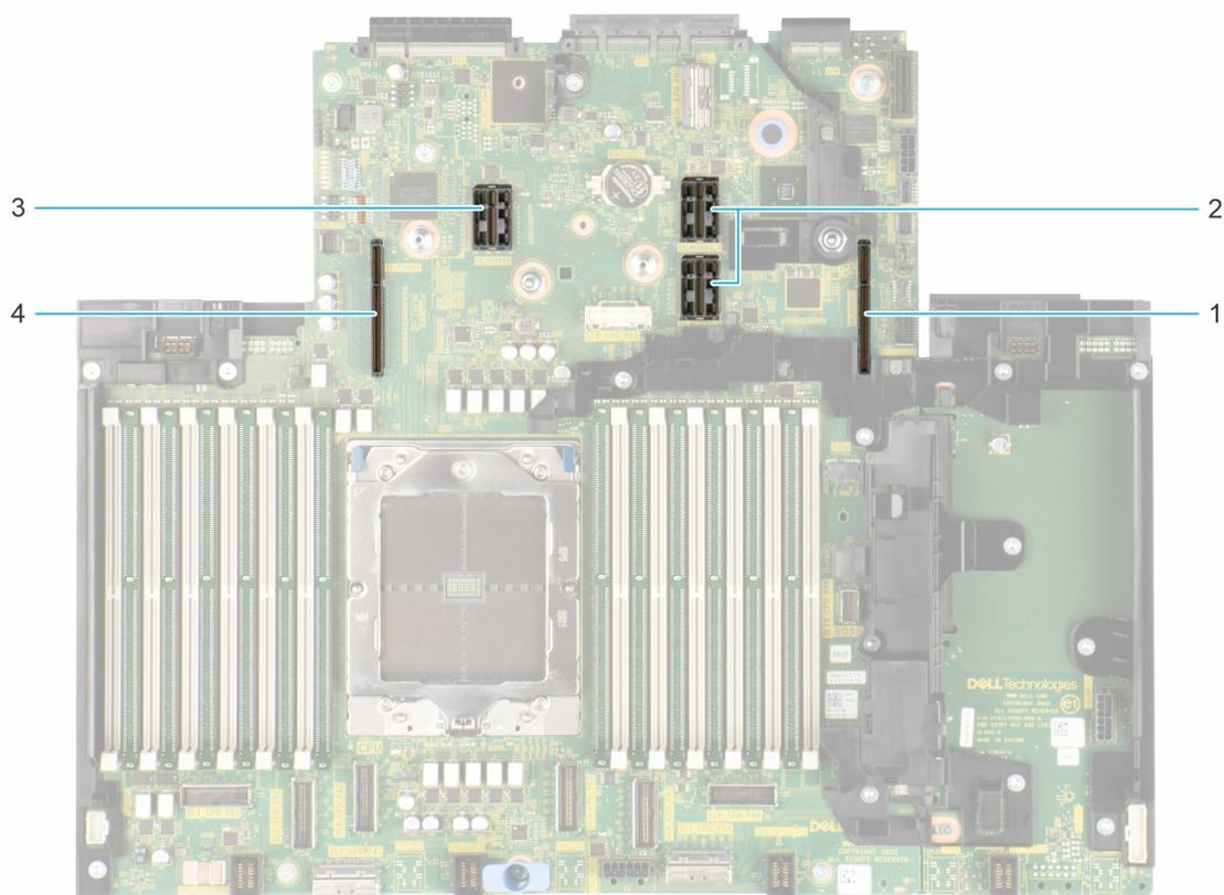
**Figure 11. Riser connector location on system board**
