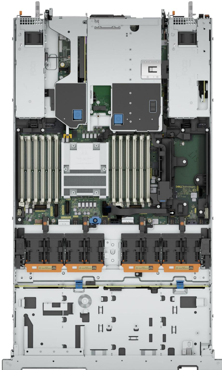
Figure 9. Inside the system with Risers + Rear 2 x E3.S
