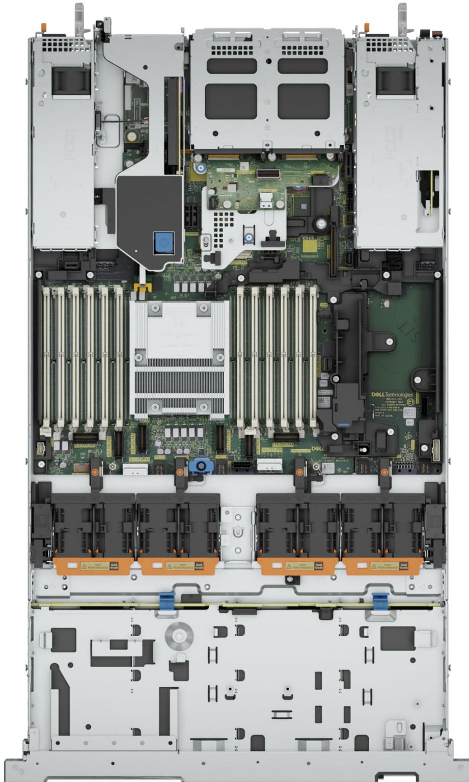
**Figure 8. Inside the system with Risers + Rear 2 x 2.5-inch module**
