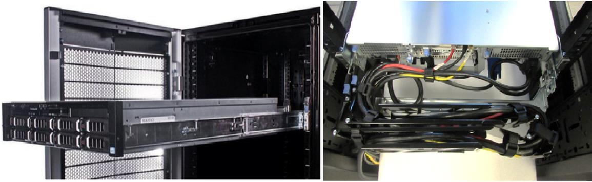
**Figure 26. Sliding rails with CMA cabling**
