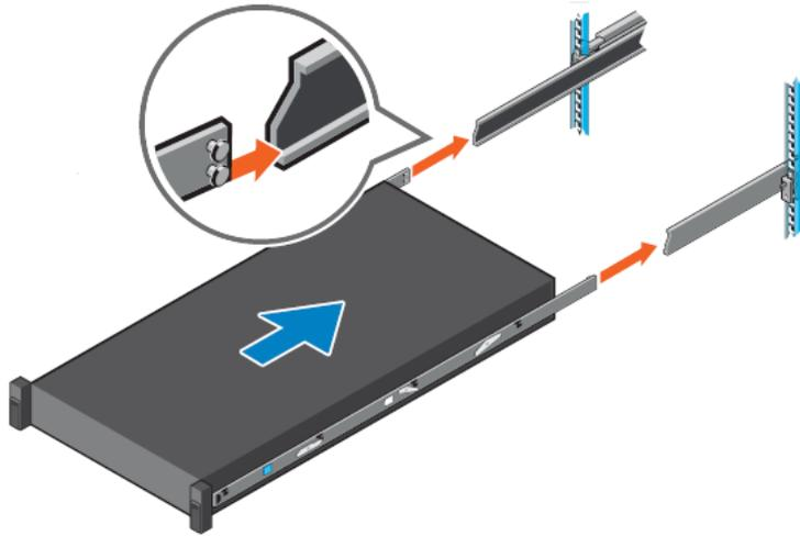
**Figure 34. Install system into the extended rails**
