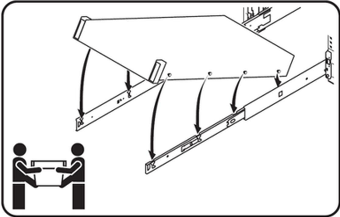
**Figure 28. Installing the system in Drop-in sliding rails**
