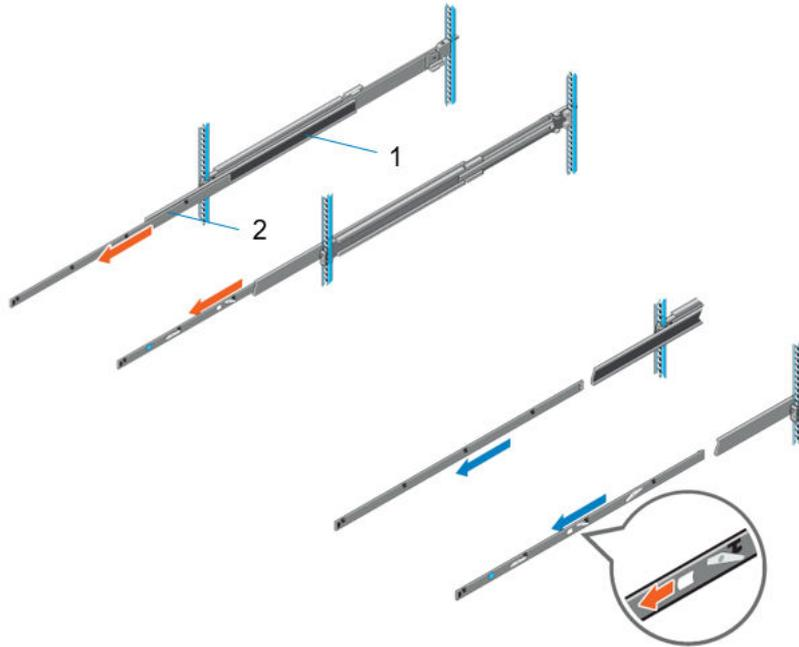
**Figure 32. Pull out the intermediate rail**
