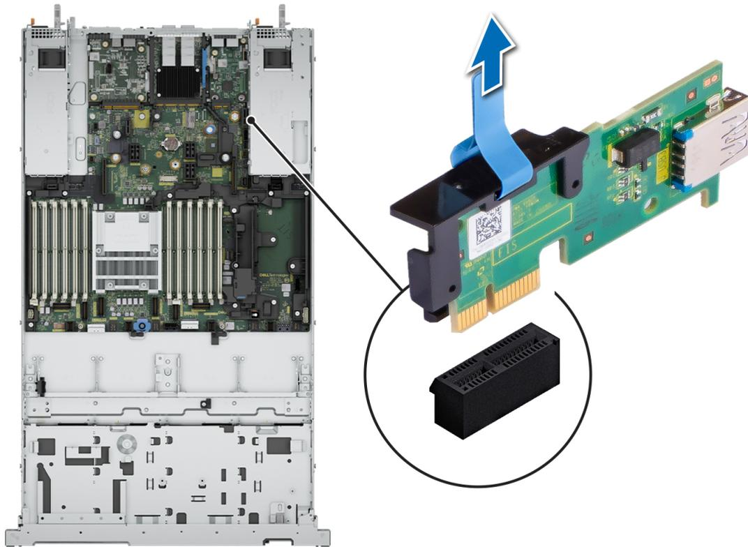
Figure 46. Internal USB Port
