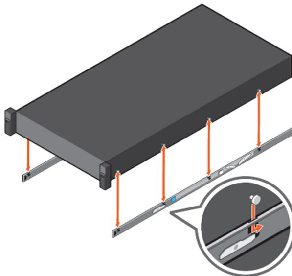
**Figure 33. Attach the inner rails to the system**
