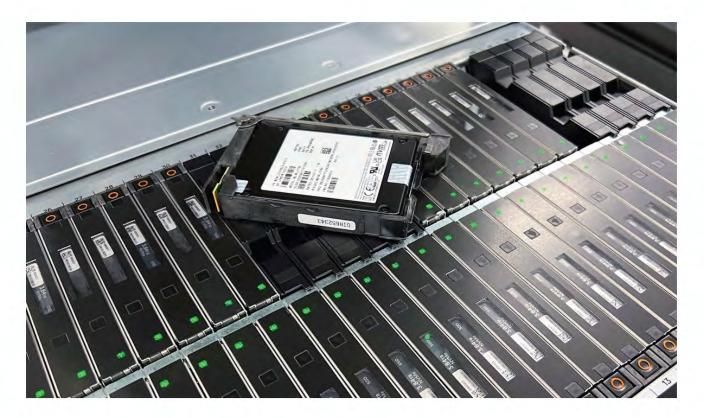
Flexible RAID provides all compute nodes in the system with active-active access to storage resources that are distributed across all DMEs. The technology reduces RAID overhead, allowing higher system capacity while using fewer drives. For example, with Flexible RAID, 1 TB can be rebuilt in less than 10 minutes.
