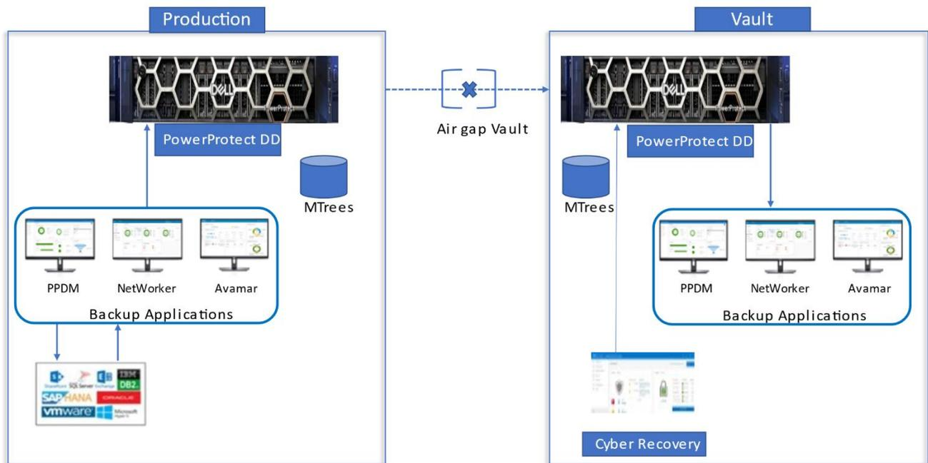
**Figure 1: Dell PowerProtect Cyber Recovery Architecture (Source: Dell)**
