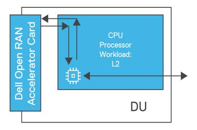
Layer 1 processing with the Dell Open RAN Accelerator Card
