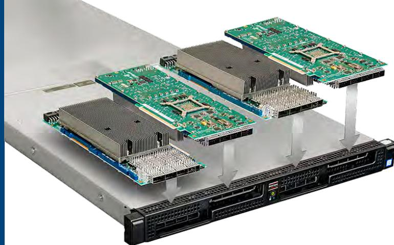
Tejeda cites as one example the BittWare TeraBox 1400DN, which is built on the Dell EMC PowerEdge C4140 server. Working directly with Dell Technologies (product engineers, assisted by OEM Solutions), his team completely re-engineered the server's chassis design to keep its 1U form factor but provide four networking interfaces on its front.
