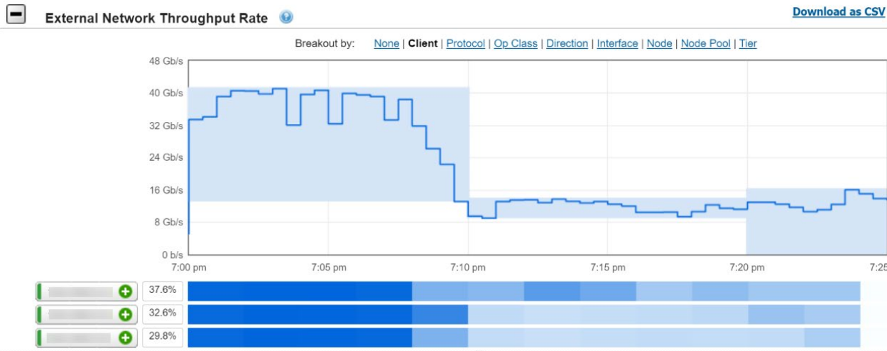
Figure 17. SSD model training storage throughput with three DGX A100 systems
