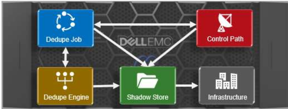
Figura 22: arquitectura modular de OneFS SmartDeduplication
