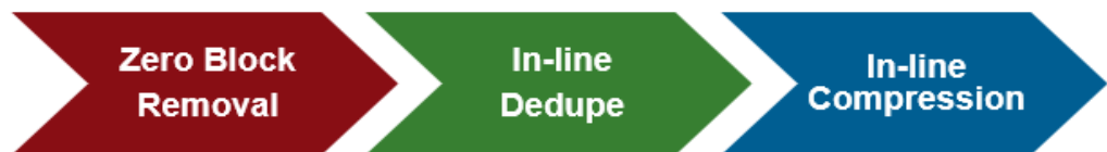
Figure 23. In-line data reduction workflow
