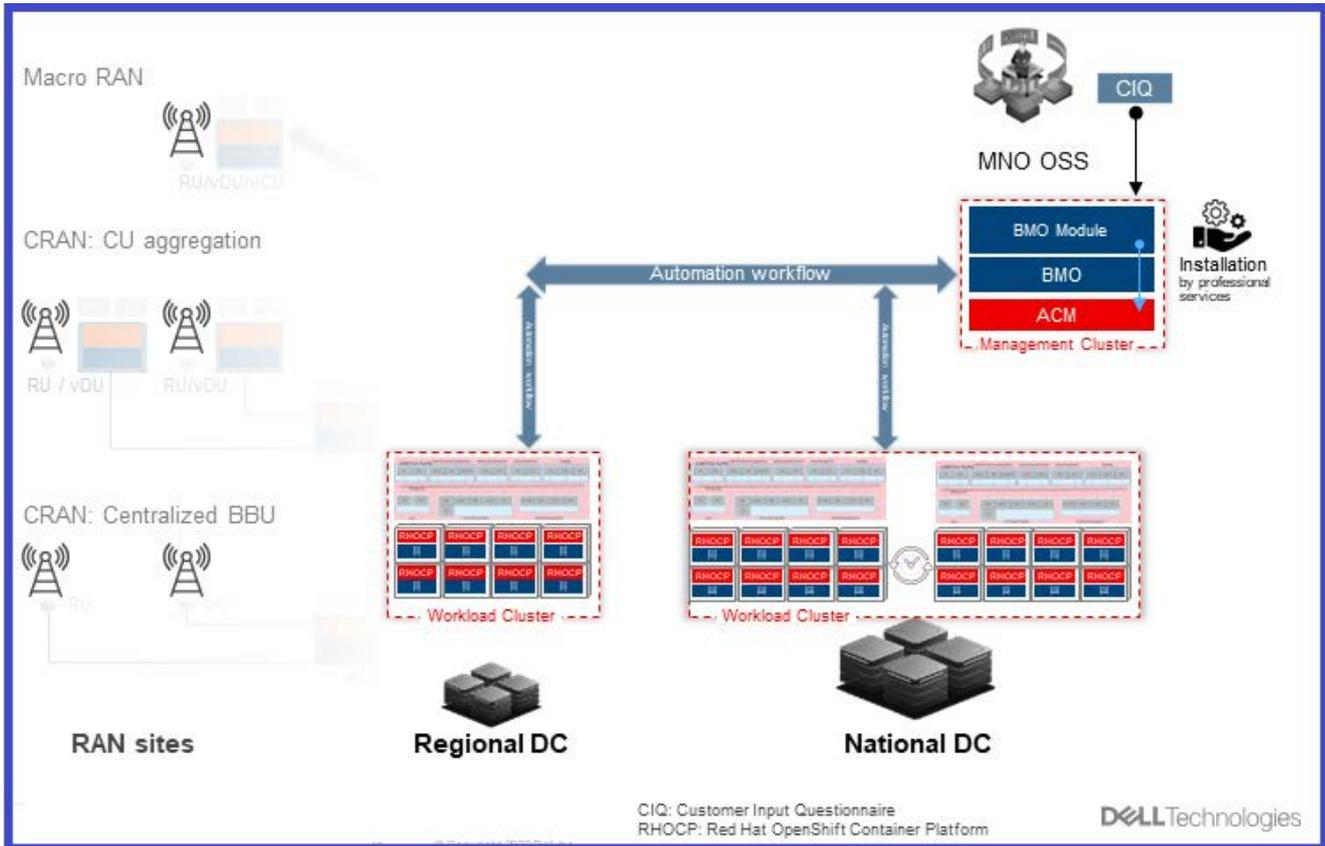
Figure 2. Telecom Infrastructure Blocks for Red Hat in a Representative CSP Deployment
