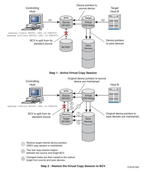
Figure 17 Incremental restore to a BCV
