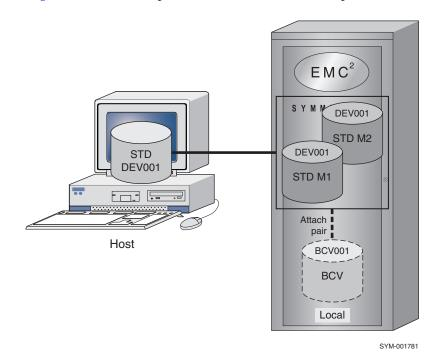
Figure 82 illustrates a preferred attachment of a BCV pair.
