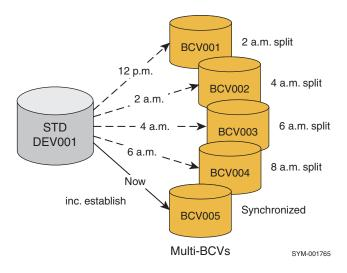
Figure 47 Establishing a multi-BCV environment
