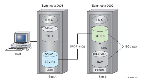
Figure 70 Restore of remote STD that mirrors local BCV
