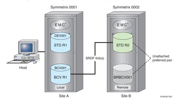
Figure 87 Detaching a BCV preference from remote STD (mirrored local BCV)
