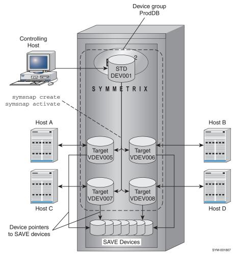
Figure 19 Creating multiple virtual copies from a standard device
