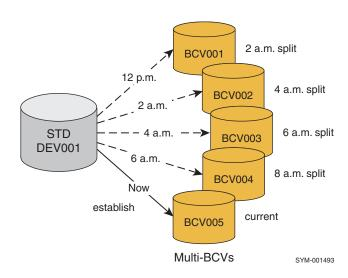
Figure 37 Establishing a multi-BCV environment
