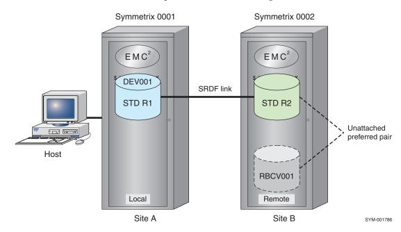
Figure 86 Detaching a BCV preference from remote STD (mirrored local STD)
