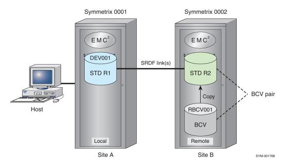
Figure 69 Full restore of remote STD that mirrors local STD
