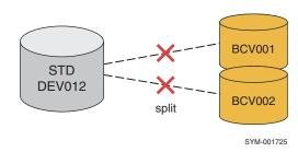
Figure 61 Splitting concurrent BCV pairs
