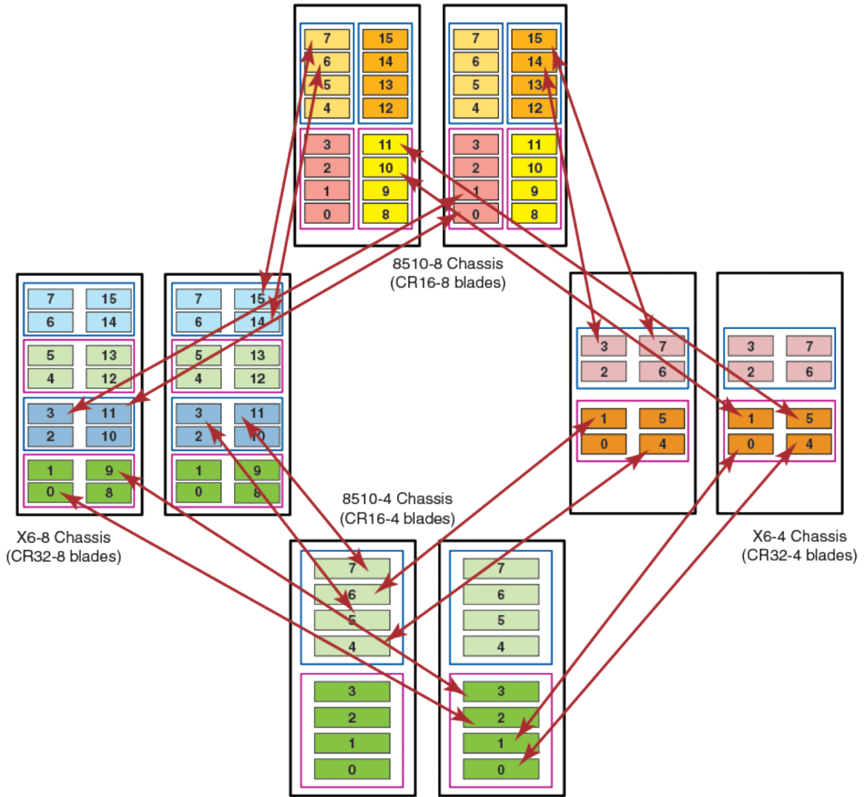
FIGURE 64 ICL trunks between DCX 8510 Backbones and X6 Directors
