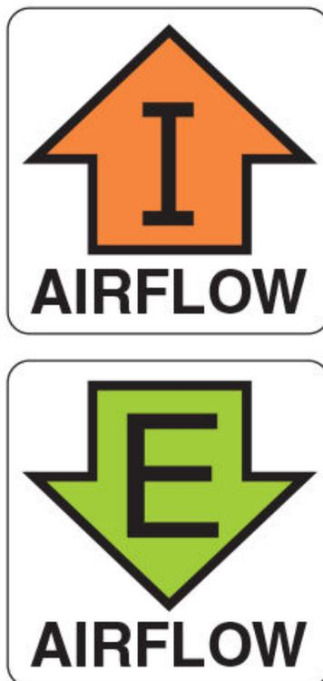
The orange **I** symbol indicates an intake FRU. This unit pulls air in from the nonport side of the device and exhausts it out the port side. This is called back-to-front airflow or intake airflow. This symbol should appear on FRUs with part numbers that contain an **NPI**.
