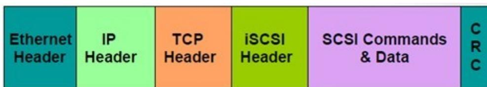
**Figure 1. SCSI commands encapsulated by Ethernet headers**
