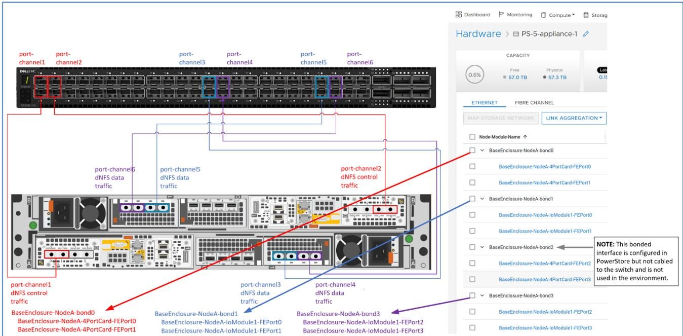
**Figure 49. Interface mappings: PowerStore and Ethernet switch**
