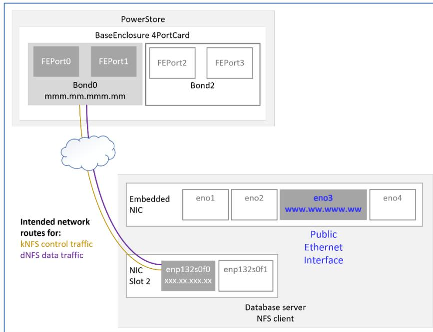
**Figure 15. Network route for dNFS traffic between the NFS client and PowerStore NAS server**
