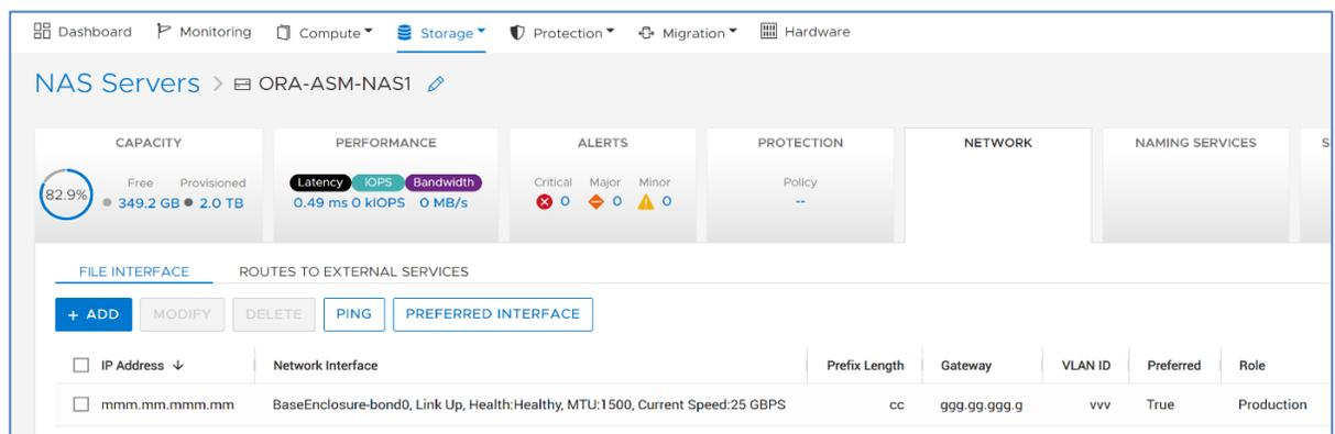
**Figure 16. PowerStore NAS server with a single bonded Ethernet network for NFS traffic**
