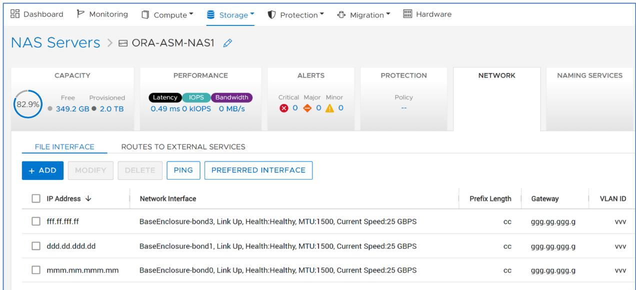
Figure 9. PowerStore bonded network interfaces
