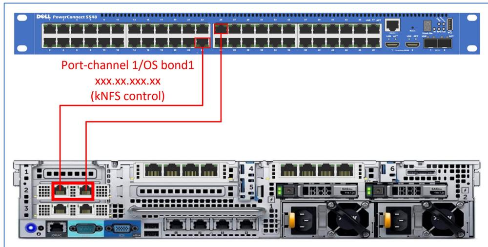
**Figure 42. Cabling bonded interfaces between the server and switch**
