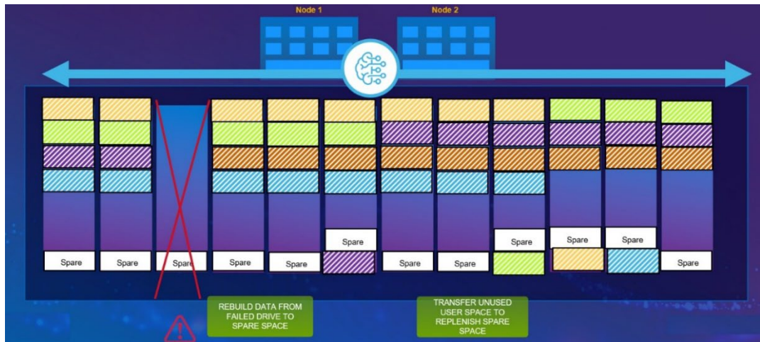
Figure 31. Rebuild data chunks to spare space after drive failure and replenish spare space with unused user space
