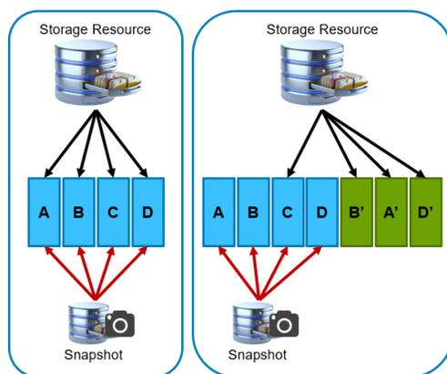
**Figure 1. Redirect-on-write example**
