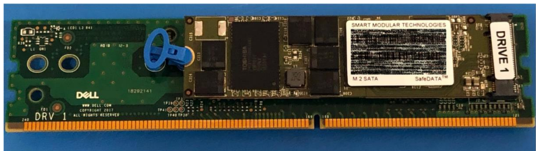
Figure 13. Internal M.2 boot module
