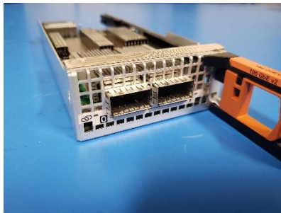
Figure 31. 100 GbE optical I/O module
