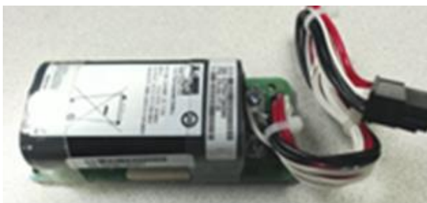
Figure 15. Battery backup unit
