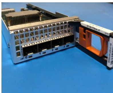
Figure 33. 32 Gb Fibre Channel I/O module
