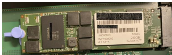
Figure 20. Internal M.2 boot module
