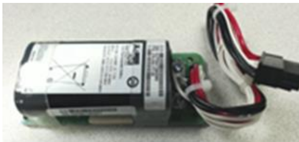
Figure 6. Battery backup unit
