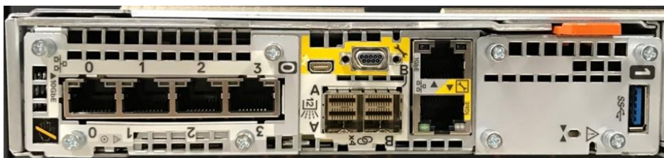
Figure 17. Embedded module with 10 GbE BASE-T 4-port card
