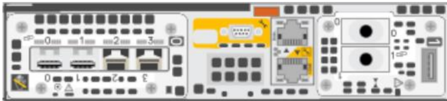
Figure 8. Embedded module with 25 GbE optical/SFP+ 4-port card
