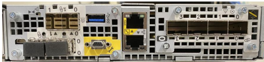
Figure 24. Embedded module with 4-port card
