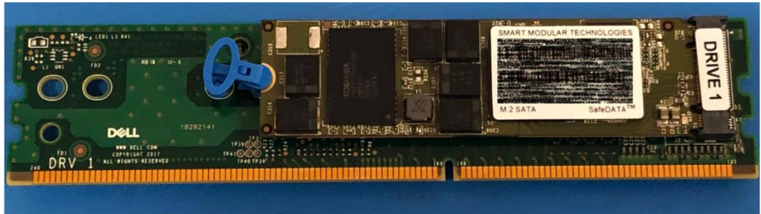
Figure 4. Internal M.2 boot module
