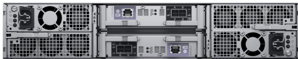
Figure 30. 25-drive 2.5-inch 2U expansion enclosure (back)
