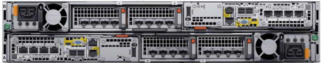
Figure 12. Base enclosure back view
