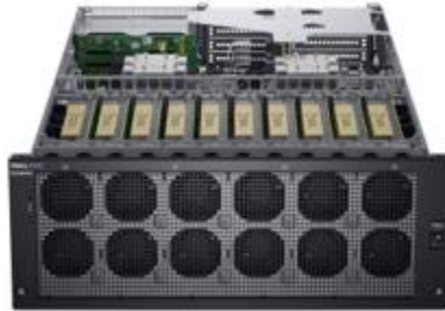
Figure 8: Dell EMC DSS 8440 server with 10 Tesla V100 GPUs
