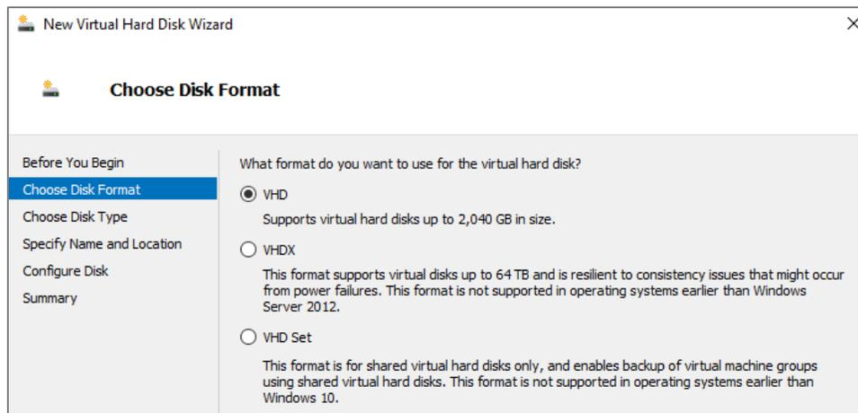
Figure 10 Different formats available for virtual hard disks
