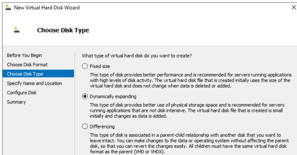
Figure 11 Select a virtual hard disk type
