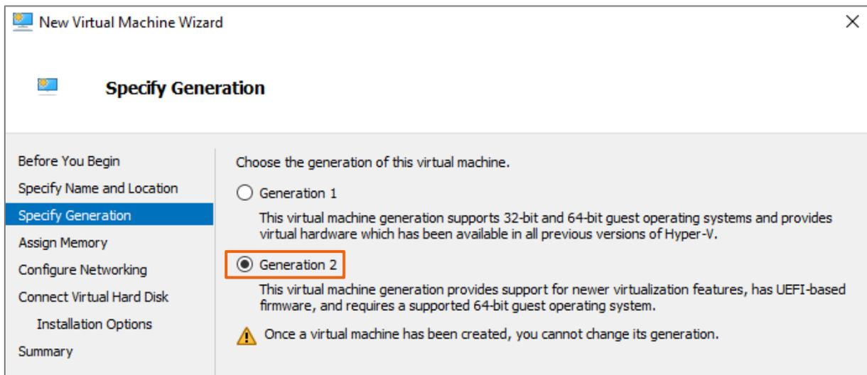
Figure 8 New virtual machine wizard in Hyper-V manager
