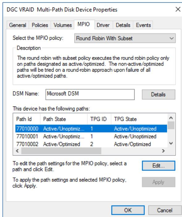
Figure 14 Verify MPIO settings (Microsoft DSM shown)
