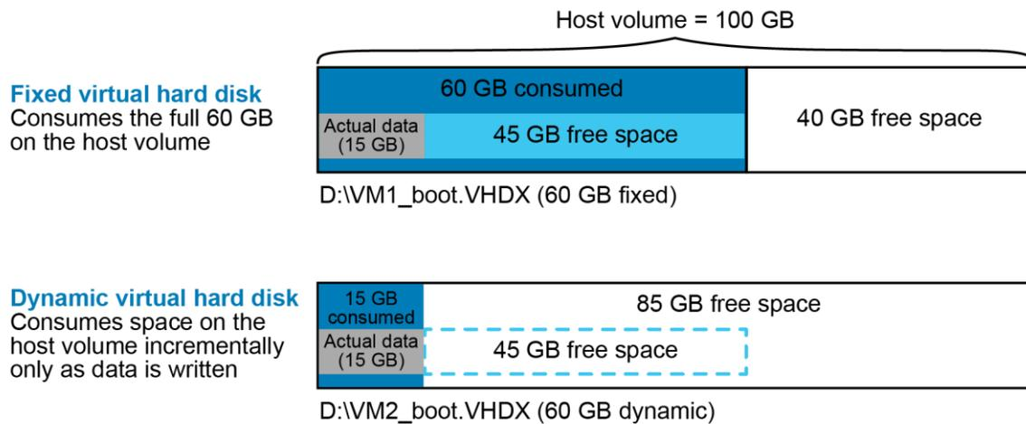
Figure 12 Fixed and dynamic virtual hard disk comparison
