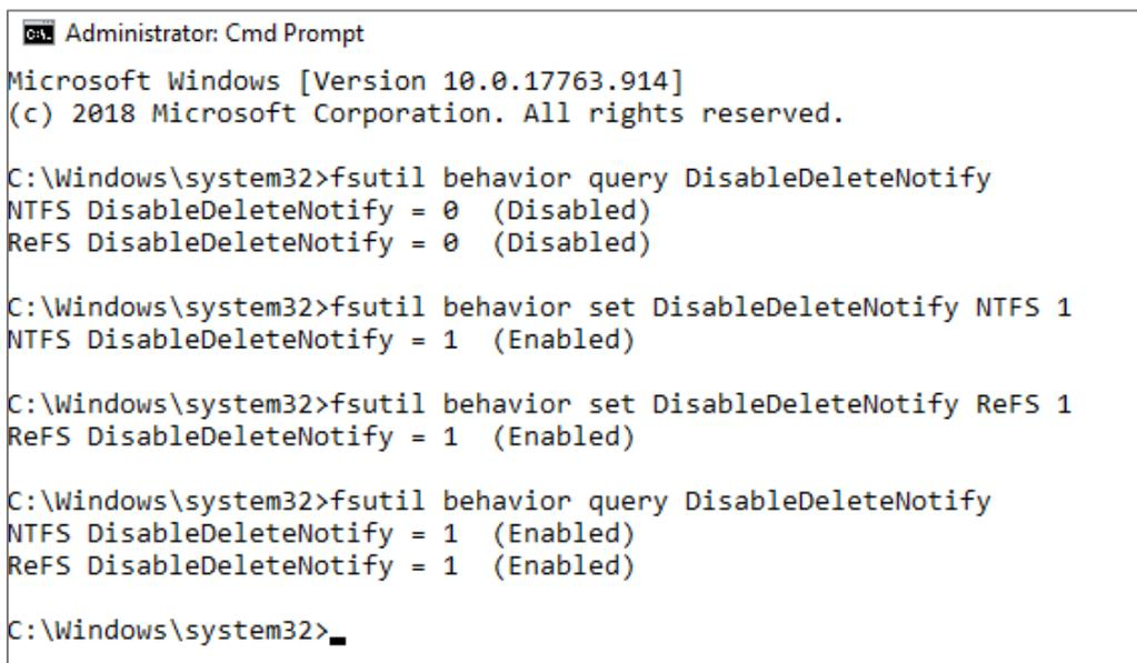
Figure 17 Use the `fsutil` command to query or change the state of trim/unmap
