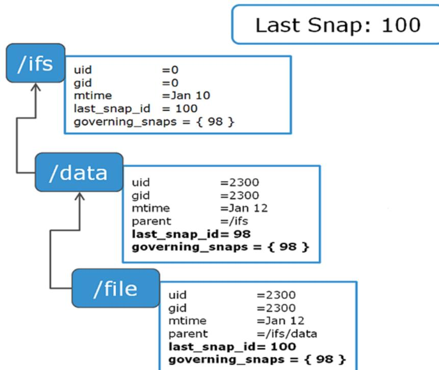
Figure 7. SnapshotIQ painting algorithm
