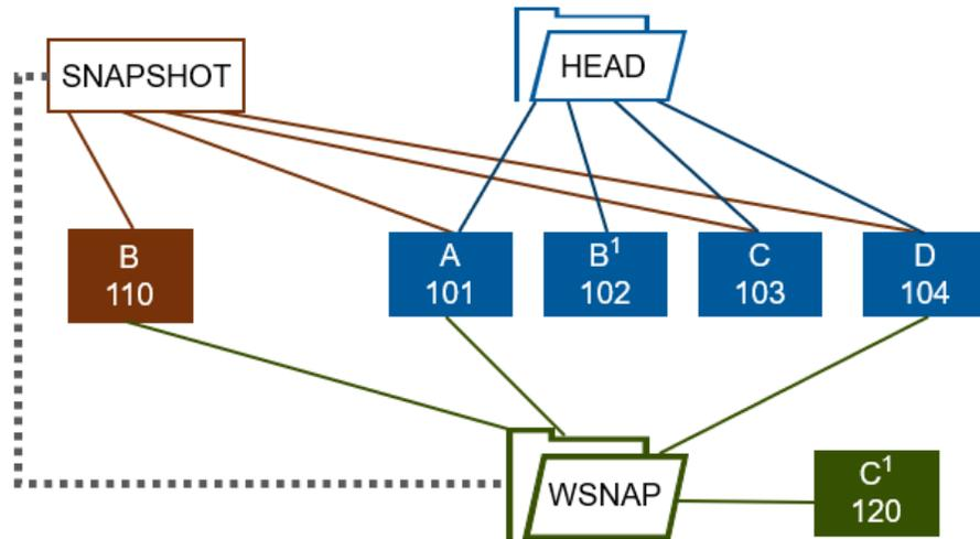
**Figure 23. OneFS writable snapshot block overlay and redirection**
