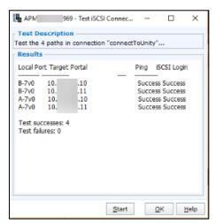
Figure 46 Test iSCSI Connection Results
