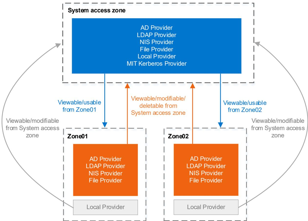
Figure 35. Authentication provider behavior in ZRBAC
