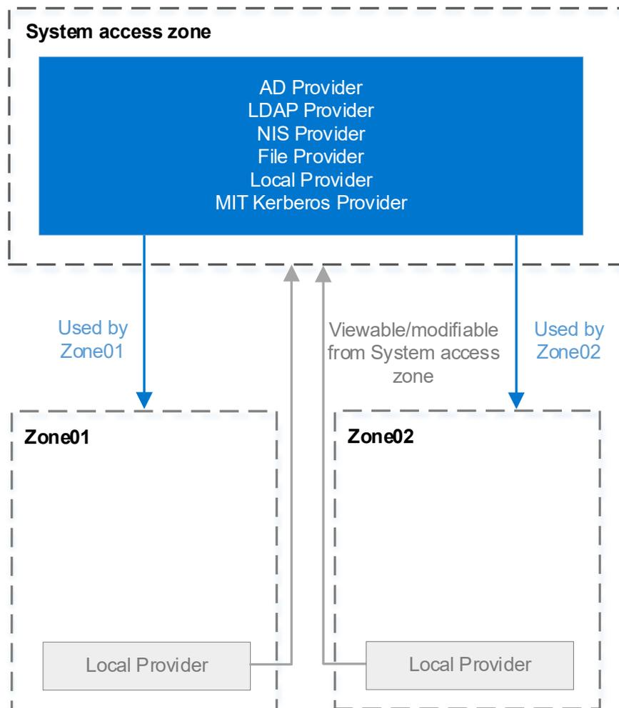
**Figure 34. Authentication provider behavior in RBAC**
