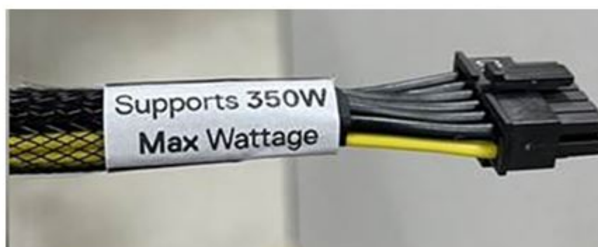
Figure 26. GPU 350 W power cable
